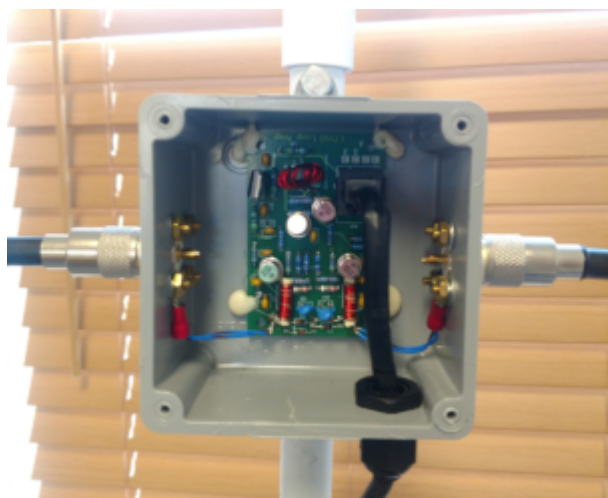
LNA mounted in box
